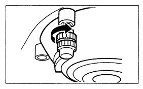
When measuring curved surfaces, if a surface with a different radius of curvature is measured, the height of the support legs should be readjusted to match the new curvature.
