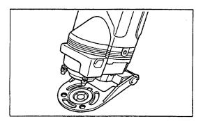
2 Tilt the Spectrophotometer so that the measurement aperture is against the specimen surface, and take a measurement.
