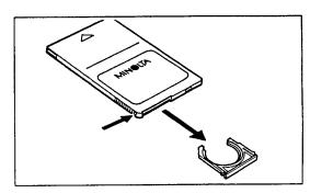
2 Remove the old battery and replace with a new CR2325 battery (or equivalent listed below) as shown at right.
