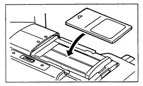
3 Slide the memory card insertion/removal slide up fully until the memory card clicks in place.
