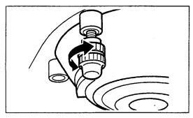
3 Turn the support leg locknut clockwise until snug to lock the support leg at the set height.
