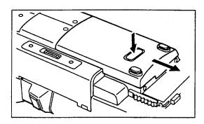
2 Pull the memory card insertion/removal slide down fully and remove the memory card.
